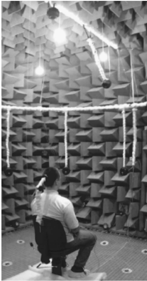
FIG. 1. The experimental setup in the anechoic chamber.
